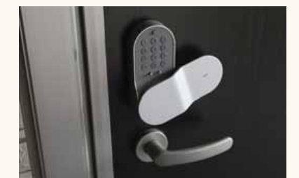
OPELO installed in a JA AMENITY HOUSE
